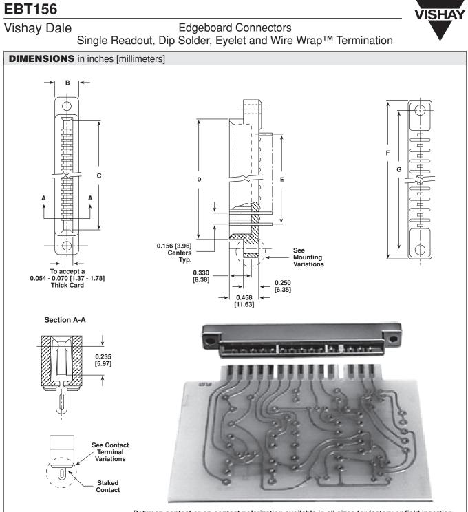
Between contact or on contact polarization available in all sizes for factory or field insertion.
